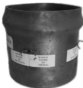
Fig. 10. Axially loaded pipe with L/D=1 after testing.
